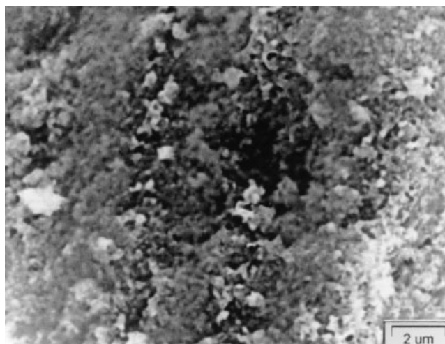
Figure 2 SEM photograph for CB after modification with Au metallic particles.
